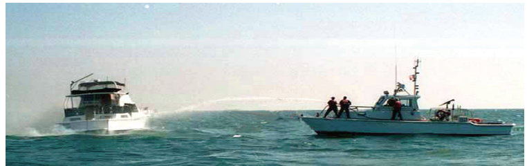
WRSS uses existing ship firefighting system.
