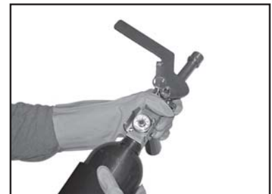
Unscrew valve and adapter.
