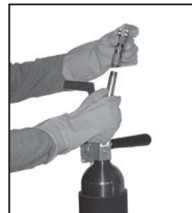
Install PepperJet filling adapter.
