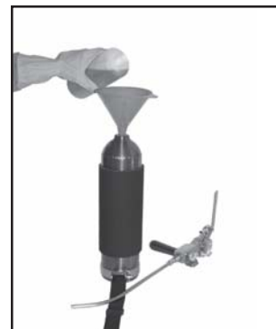
Pour refill solution into cylinder using funnel.
