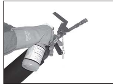
Use Leak Detector to check for leaks.
