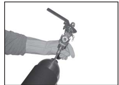
Remove valve and drawtube.
