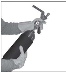
Screw valve assembly into bottle.
