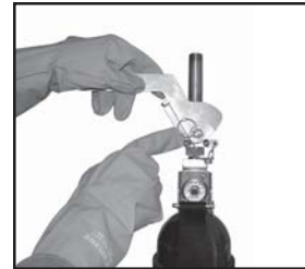
Safety chain installed.
