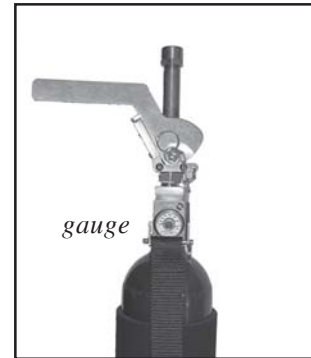
Monitor pressure gauge.
