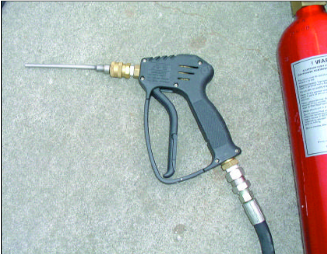
The “pressure washer” style spray handle allows for excellent control and maneuverability.
